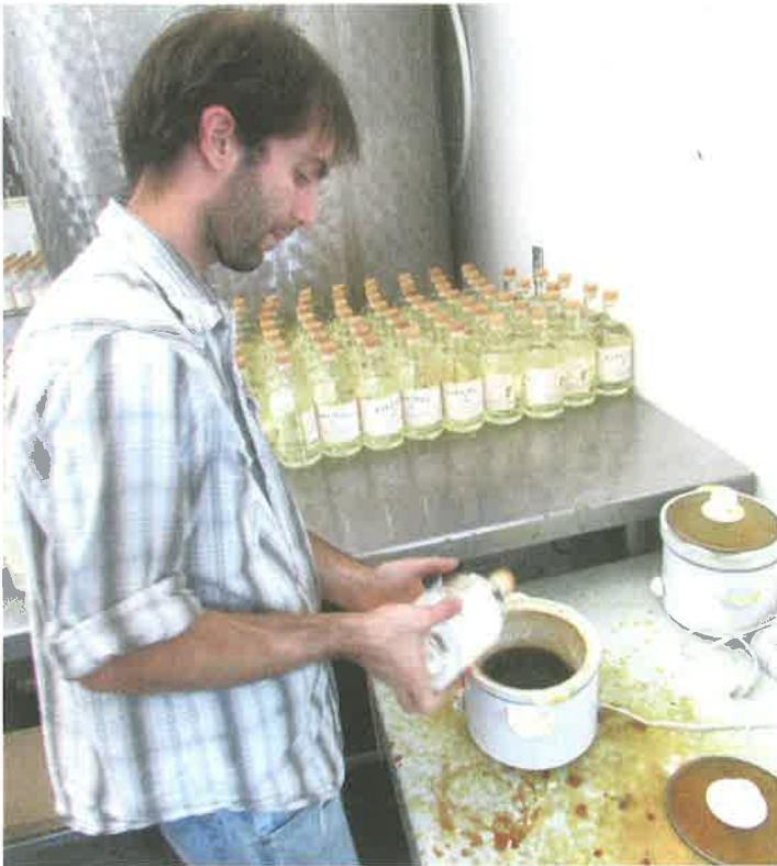
Facing page top: Head distiller Ryan Christensen stands with the Barr Hill stills, which were made from converted dairy tanks. Lower: Bottles of Barr Hill Gin lined up in front of a yellow lump of beeswax, which is melted and used to seal the bottles. Above: Production assistant Adam Mitchell dips the bottles into hot beeswax to create a fragrant seal.
